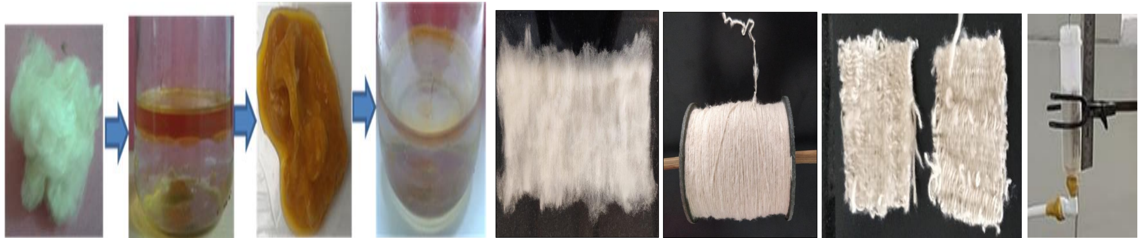
Phyto fibre Water + oil emulsion Phyto fibre adsorbs only oil
